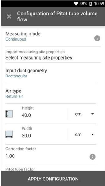
Configuration of Pitot tube volume flow
