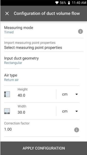
Configuration of duct volume flow
