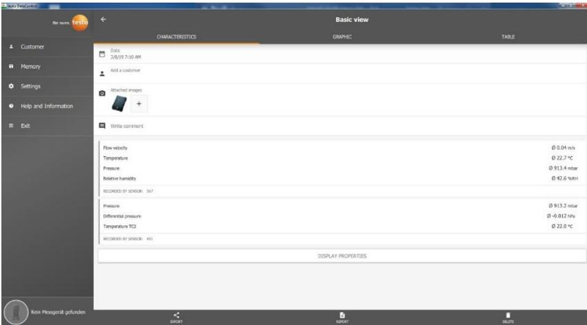
The measurement results listed are divided into three areas. • Display of the calculated results of the application menu
