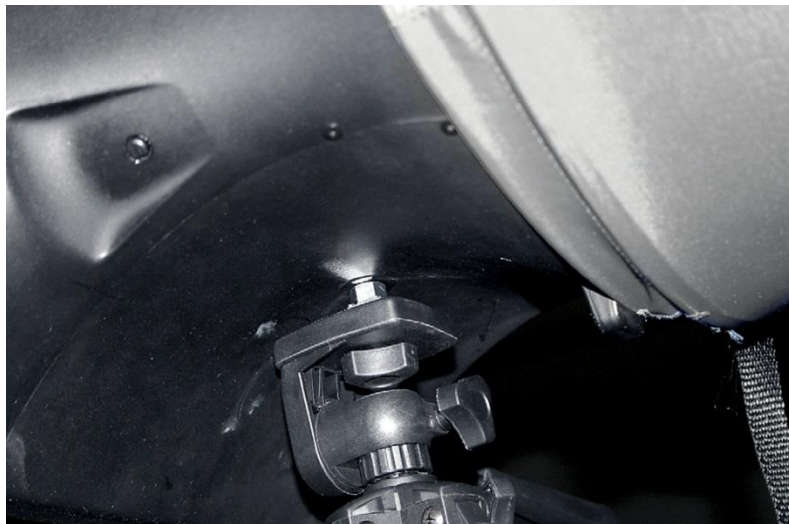
Figure 27: Mount Hood Base to Telescopic Stand
