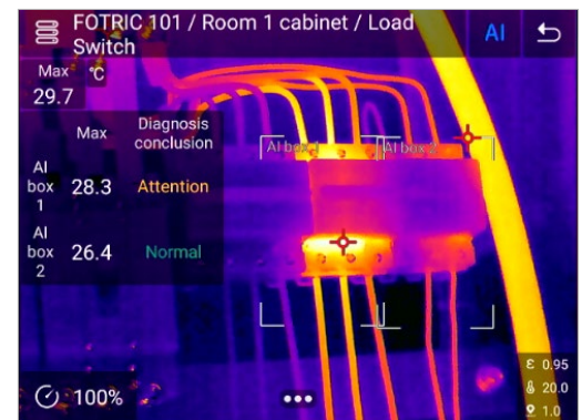
NaviPdM on-device ROI-based alarms
